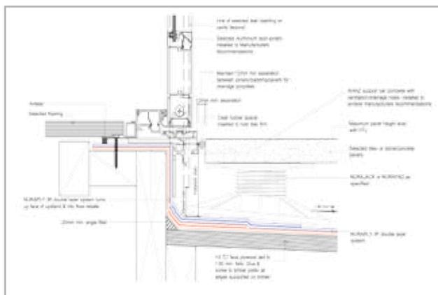
Frameless Balustrade Timber Decking on Aluminium Tube
